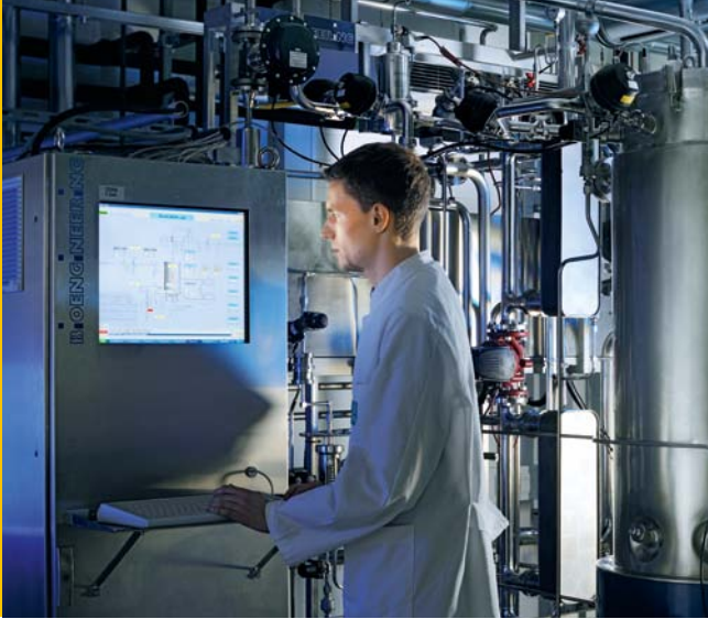
The 300-liter bioreactor plant is used for microbial cultivation.
